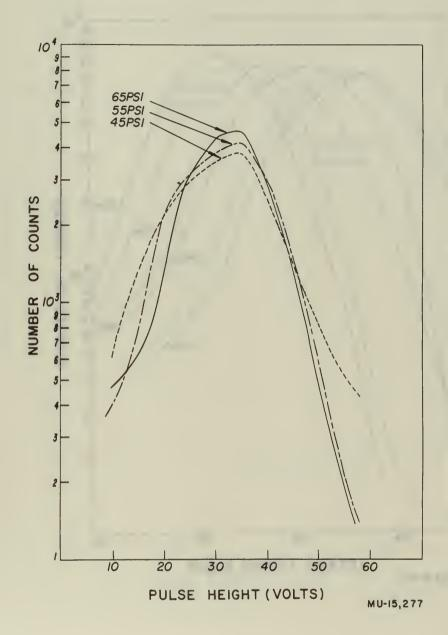
Fig. 6. Pulse height spectra for increasing pressure in argon at 22° C. Cm<sup>244</sup> source.
